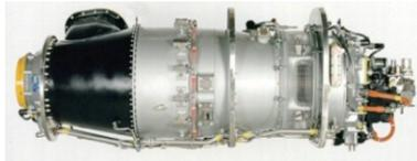
Fig. 7. PWC PT6A-62 turboprop engine
